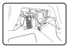
2: Remove 5 screws & 2 hex head bolts from 4: Dispose of used filter correctly. around glove box frame, gently pull glove box out until plug for glove box light is visible and disconnect, Remove glove box to expose cover for cabin filter. Remove cover to gain access to filter by pulling out.
